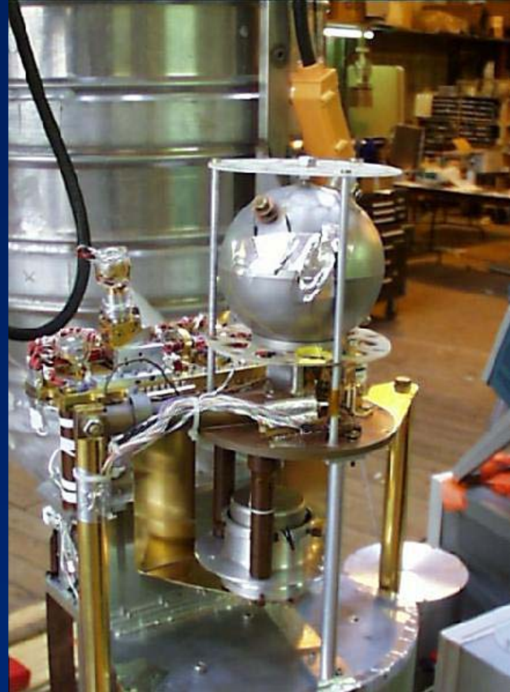
The He3 refrigerator for BOOMERANG
