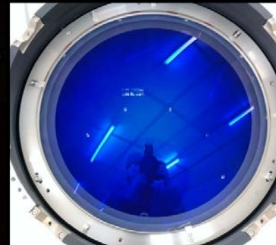
L2: 50 mm thick, 300 mm diameter aspherical lens.
