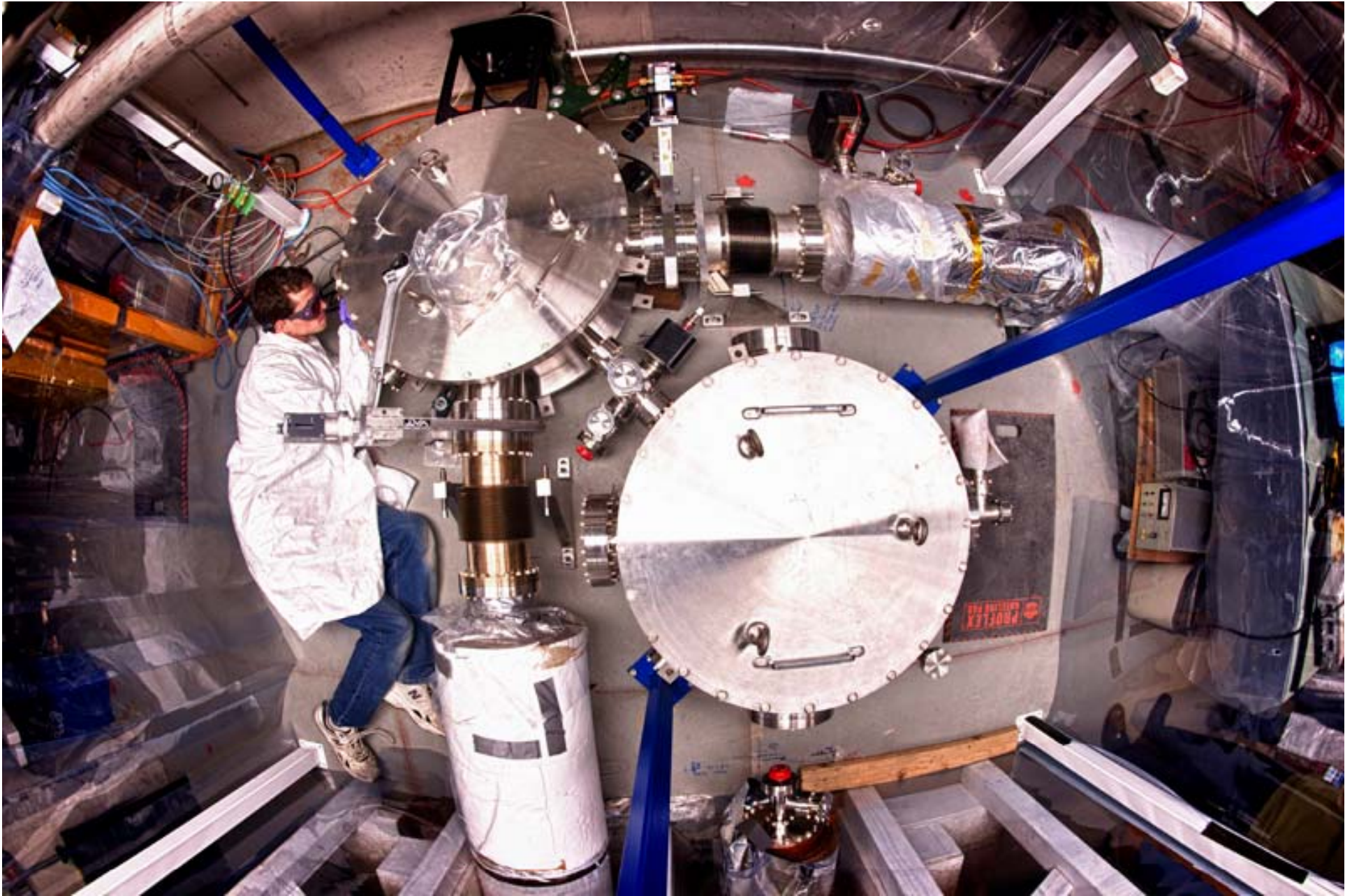
Ben Brubaker bolting the holometer vacuum system together
