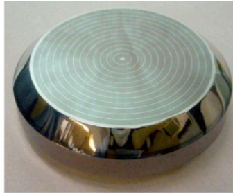
ID2 to ID5: Φ 70mm, H 20mm, 410g 13 concentric electrodes (width 200μm for ID2, 50 μm for ID3, spacing 2mm) with bevelled edge 8 mm.
