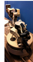
Fig. 1: Measurement setup of the TMBi refraction index. A prismatic cell filled with water is placed at the center of the goniometer plateau for a systematic check.
