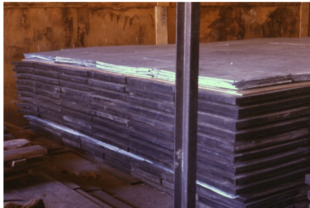
Рисунок 3: Emulsion experiment on the city of Chakaltaya (Andes, Bolivia). Unique characteristics of the setup - the height of the location (4370 m above sea level); the world's largest ( \sim 1000 \text{ m}^2 ) solid-state tracking camera with high spatial resolution ( \sim 10 microns) and with a high threshold for particle registration ( \sim 4 \text{ TeV} )
