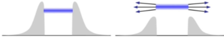
Figure 3: Centrifugal barrier for particles with different masses: left – light mass, right – heavy mass.
