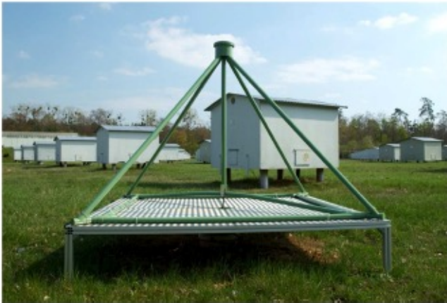
(a) Inverted v-shape dipole at LOPES
