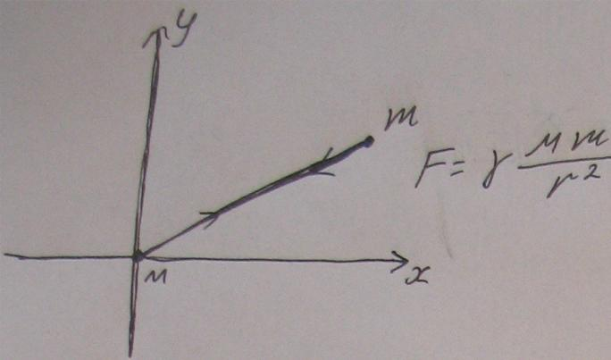
$$\vec{F} = -\gamma \frac{Mm\vec{r}}{r^3} = \left(-\gamma \frac{M}{r^3} \vec{r}\right)m = \vec{G}m$$
